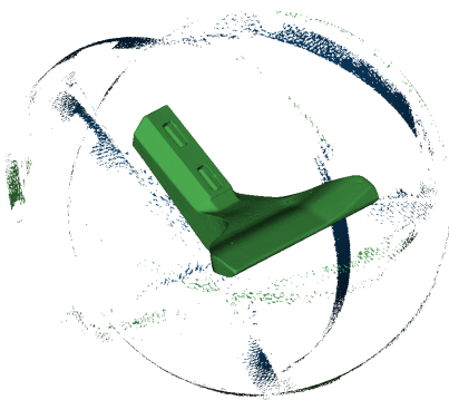
A model with rims of a turntable. None of the stray parts are touching the object.
